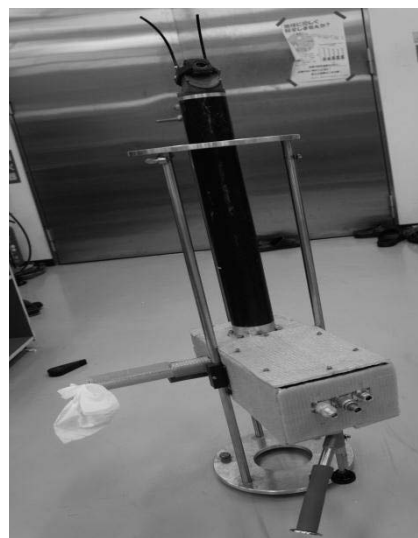
Figure1:A photograph of the second prototype of cryocoil MAS probe
