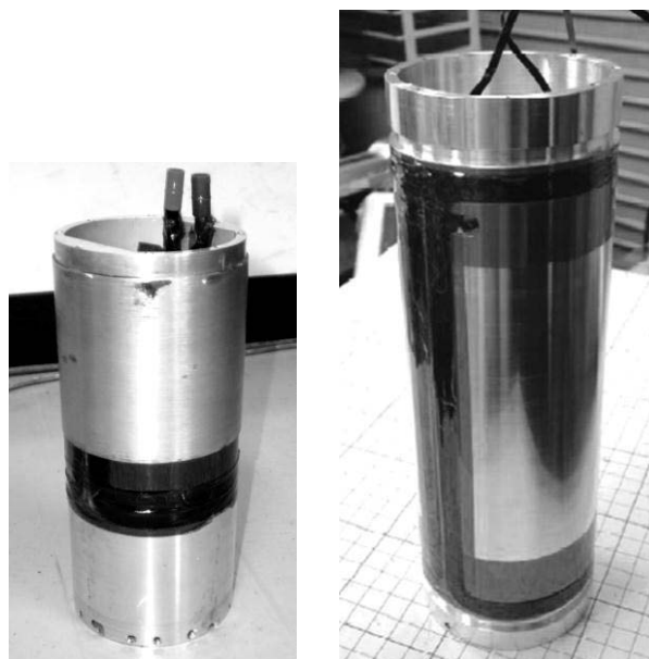
Fig. 1 Pictures of X_0 shim coils. Left; the 2 nd prototype: coil size \phi 71 \text{ mm} \times 90 \text{ mm} . Right; the 3 rd prototype: coil size \phi 72 \text{ mm} \times 172 \text{ mm} .
