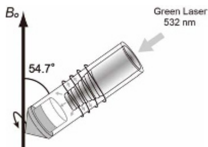
Fig. 1 The schematic of in situ photo-irradiated solid-state NMR.
