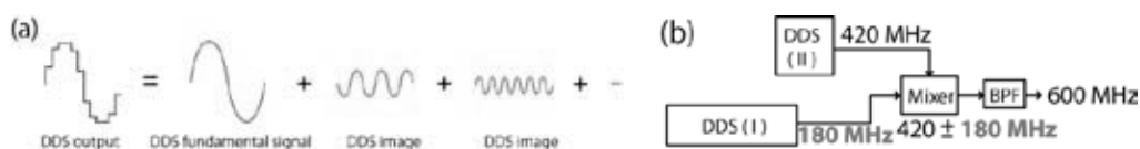
Fig. 2. (a) A schematic figure that DDS output is a superposition of a fundamental signal and image signals. (b) A scheme to generate a RF signal at 600 MHz using the DDS image at 180 MHz instead of the DDS fundamental signal at 20 MHz.
