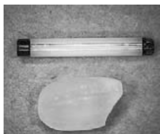
Fig.1 1mmΦ rotor for high speed MAS and rice grain.
