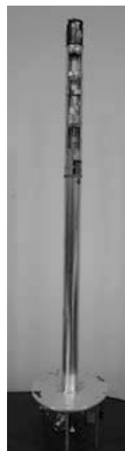
Fig.2 1mm MAS probehead for 800 MHz instrument
