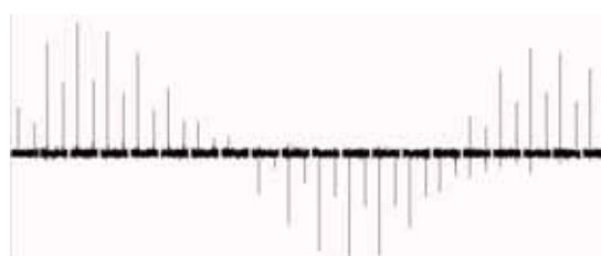
Fig.1(b) ^{13}\text{C} pulse nutation of adamantane from 0.2 \mu\text{s} to 4.0 \mu\text{s} (left to right) at 180W.
